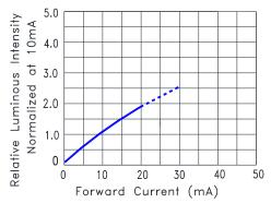
Fig.4 Relative Luminous Intensity vs. Forward Current
