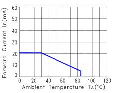
Fig.2 Forward Current Derating Curve
