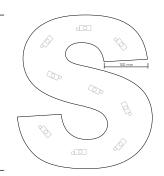
Height: 350 mm Stroke: 100 mm Depth: 70 mm Brightness: ~1750 lx Typeface: Arial Black
