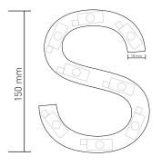
Height: 150 mm Stroke: 18 mm Depth: 40 mm
