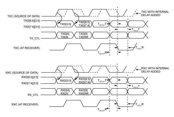
Figure 14. RGMII v2.0 Specification (Figure3-Multiplexing and Timing Diagram)
