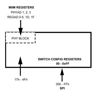
Figure 12. Interface and Register Mapping
