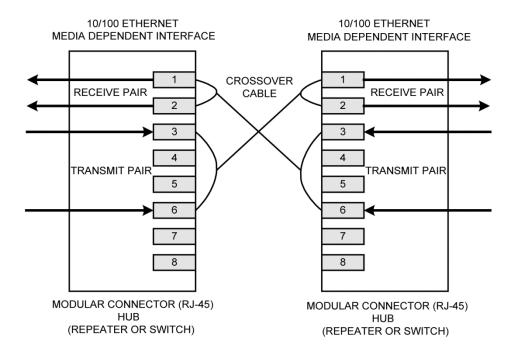
Figure 2. Typical Crossover Cable Connection
