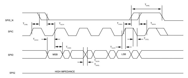
Figure 21. SPI Input Timing
