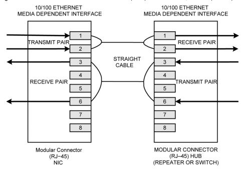
Figure 1. Typical Straight Cable Connection
