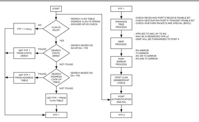
Figure 4. Destination Address Lookup and Resolution Flow Chart
