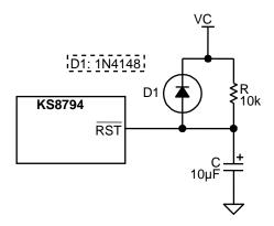
Figure 25. Recommended Reset Circuit
