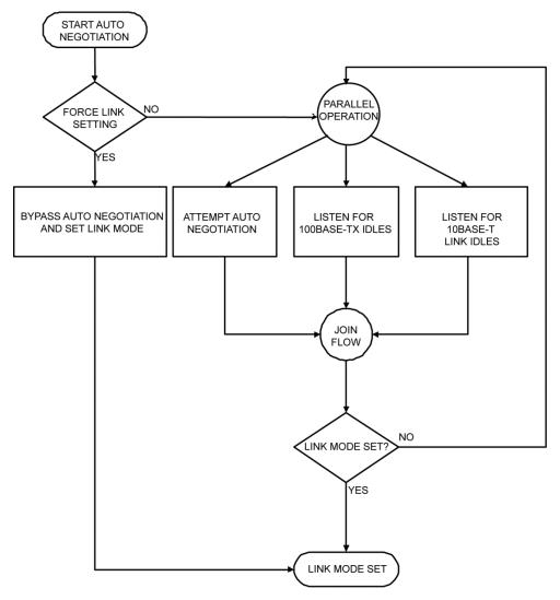
Figure 3. Auto-Negotiation and Parallel Operation
