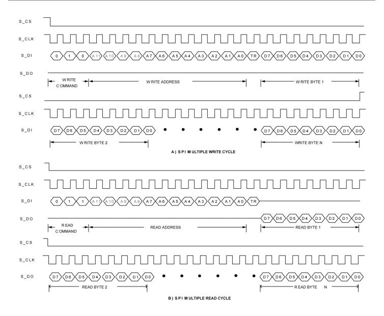
Figure 8. SPI Multiple Access Timing
