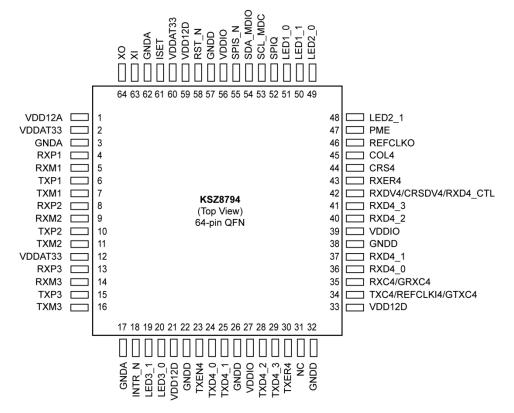
64-Pin QFN Pin Configuration
