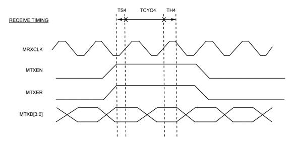
Figure 17. PHY Mode MII Timing – Data Received from MII
