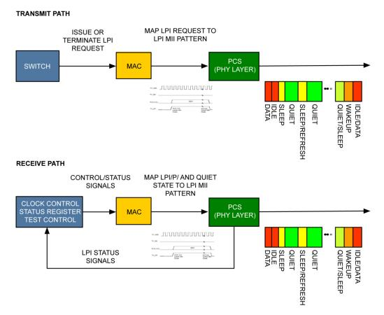
Figure 5. EEE Transmit and Receive Signaling Paths
