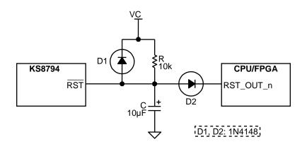
Figure 26. Recommended Circuit for Interfacing with CPU/FPGA Reset
