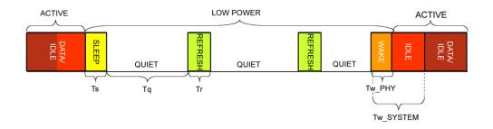
Ts = THE PERIOD OF TIME THAT THE PHY TRANSMITS THE SLEEP SIGNAL BEFORE TURNING ALL TRANSMITTERS OFF,  $200 \le Ts \le 220$  USED IN 100BASE-TX. Tq = THE PERIOD OF TIME THAT THE PHY REMAINS QUIET BEFORE SENDING THE REFRESH SIGNAL,  $2000 \le Tq \le 22000$  USED IN 100BASE-TX. Tr = DURATION OF THE REFRESH SIGNAL,  $200 \le Tr \le 220$  USED IN 100BASE-TX.
