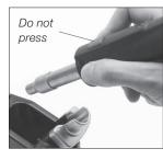
The tool automatically starts blowing hot air when lifted from the stand.
