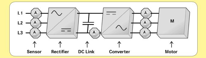
• Frequency converter for Generator-Grid connection
