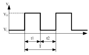
$$T = \frac{1}{f_{\text{PWM}}} = t1 + t2(\text{sec}) \quad . \label{eq:T_pwm}$$
