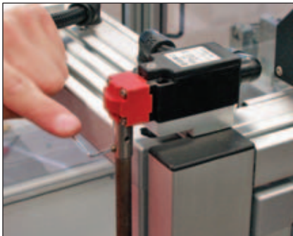
Temporary shaft locking (dowel provided).
