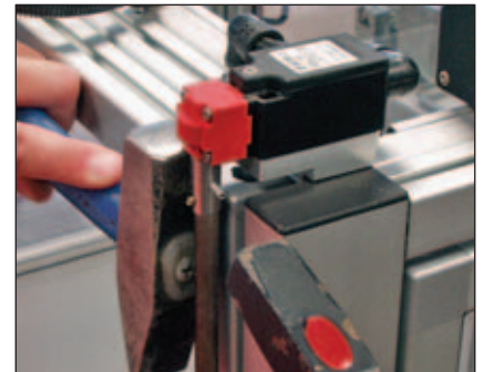
Switch locking (pin provided).
