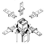
The head can be quickly rotated on each of the 4 sides of the switch by unfastening the two fixing screws. The mechanical delay device can be rotated in 90° steps as well. This enables the switch assume 32 different to configurations.
