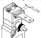
This switch has a wide backlash of the actuator into the head (4.5 mm) for an easier installation.
