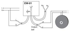
2. The device connected to the existing bell system.
