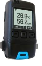
The EL-GFX-2 standalone USB data logger measures and stores up to 252,928 temperature and humidity readings over a -30 to +80°C (-22 to 176  $^\circ\text{F})$  and 0 to 100%RH range at a resolution of 0.1  $^\circ\text{C}$  and 0.1%RH.
