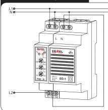
Control and L1 phase voltage drop signalling circuit.
