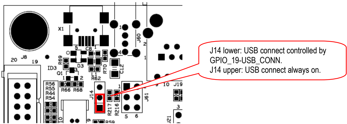
Figure 42 – Jumper Setting: USB Connect, J14
