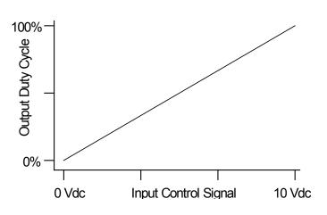
Figure 1: Default Analog 0-10 Vdc Control Curve
