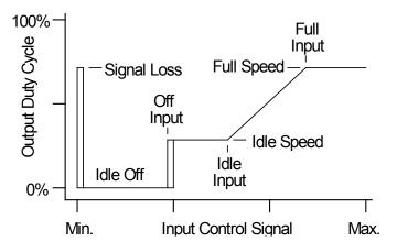
**Figure 4:** ECM-Motor Speed vs. Input Signal Configurable Options
