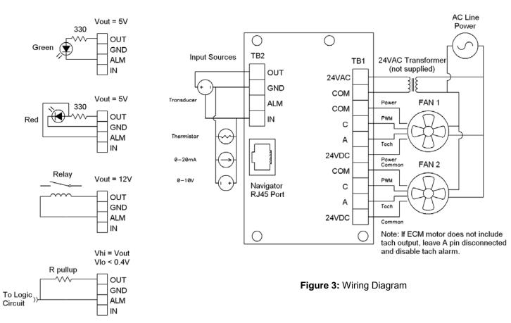
Figure 2: Alarm Configuration Examples
