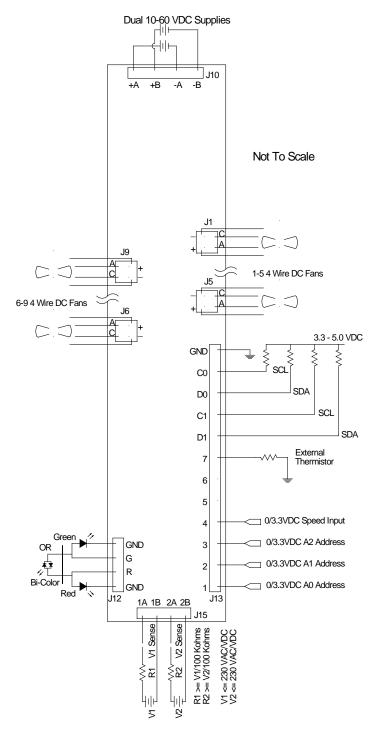
**Figure 2.0**: Connection diagram showing input power, fan, interface, temperature sensor, LEDs and alarm connections for a Cirrus-9 Fan Control.
