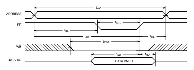
Figure 10. Write Cycle No. 3 (WE Controlled, OE LOW) [27, 30]
