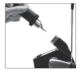
When the tool is lifted from the stand the tip will heat up to the selected temperature.
