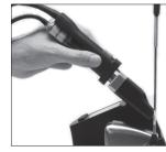
When the tool is in the stand, the temperature falls to Sleep temperature (pre-set 260°C / 500°F).
