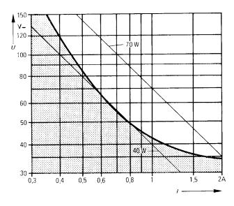
/ = switching currentU = switching voltage
