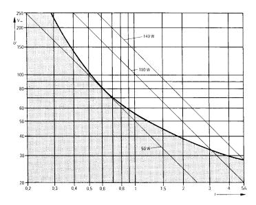
Safe breaking, no stationary arc Contact material silver, gold-flashed
