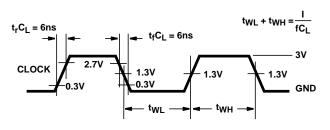
NOTE: Outputs should be switching from 10% V<sub>CC</sub> to 90% V<sub>CC</sub> in accordance with device truth table. For  $f_{MAX}$ , input duty cycle = 50%.
