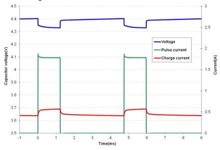
Fig 5 shows that the GS203 supercapacitor does an excellent job supporting a GPRS class 10 pulse train, drawing 1.8A for 1.1ms at 25% duty cycle. The source is current limited to 0.6A and the supercapacitor provides the 1.2A difference to achieve the peak current. At first glance the freq response of Fig 8 indicates the supercapacacitor would not support a 1ms pulse, but the Ceff of 78.3mF coupled with the low ESR supports this pulse train with only ~70mV droop in the supply rail.
