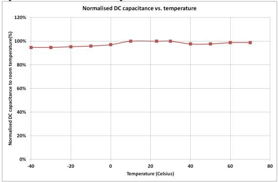
Figure 6: Capacitance change with temperature
