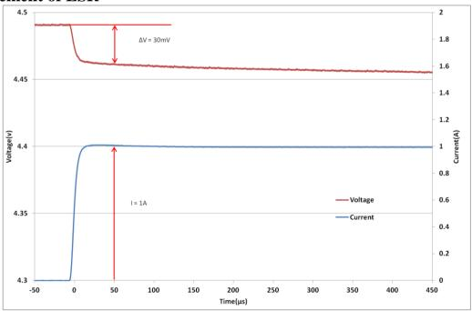
Fig 3: Measurement of ESR for a GS203
