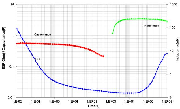
Fig 9: Frequency Response of ESR, Capacitance & Inductance
