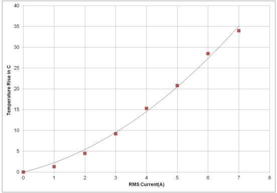
Fig 12: Temperature rise in GS203 with RMS current
