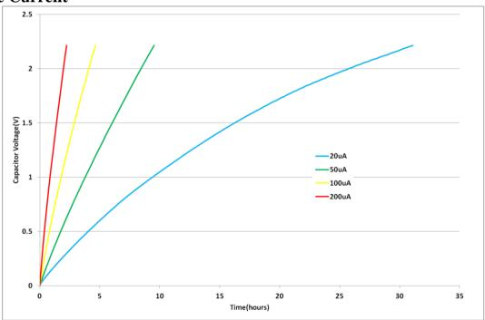
Fig 11: Charging a GS103 with low current
