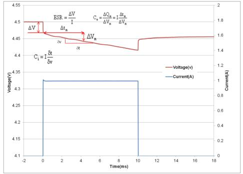
Figure 1: Effective capacitance, instantaneous capacitance and ESR for a GS203
