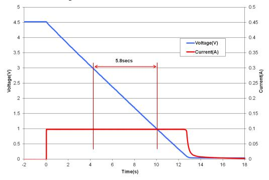
Fig 2: Measurement of DC Capacitance for a GS203
