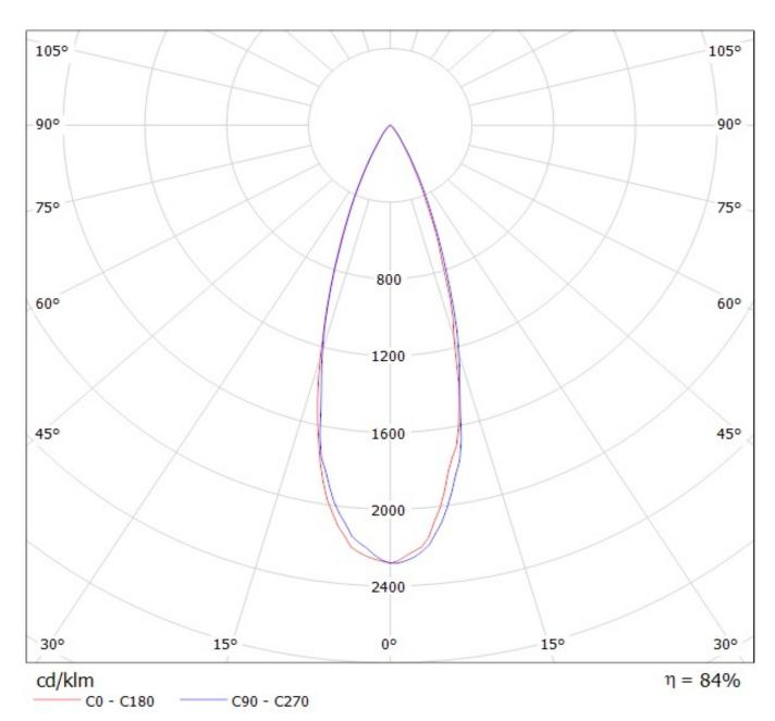
Luminaire: Ledil Oy CA11355\_Laura-M\_(XP-G2) Efficiency=83% Lamps: 1 x Cree XP-G2 (XPGBWT-L1-0000-00FE4) 102Im @ 250mA CCT=4900K P=0.8W I=250mA
