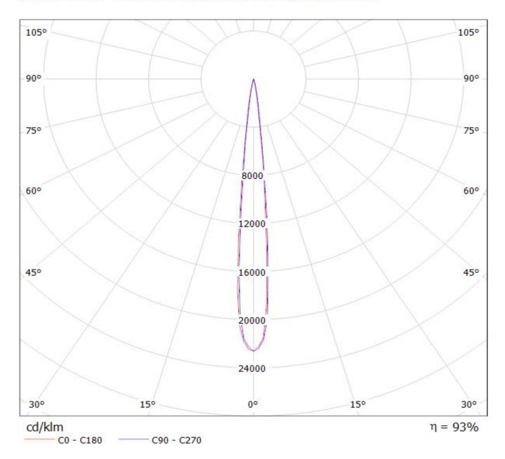
Luminaire: Ledil Oy CA11353\_LAURA-RS\_(3535\_Ceramic\_gen2) Efficiency=89% Lamps: 1 x LG 3535 Ceramic gen2 (PKG5700K) 116Im @ 250mA CCT=6200K P=0.7W I=250mA
