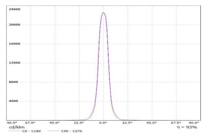
Luminaire: Ledil Oy CA11353\_LAURA-RS\_(3535\_Ceramic\_gen2) Efficiency=89% Lamps: 1 x LG 3535 Ceramic gen2 (PKG5700K) 116Im @ 250mA CCT=6200K P=0.7W I=250mA
