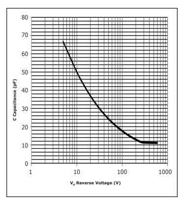
Figure 4. Capacitance vs. Reverse Voltage
