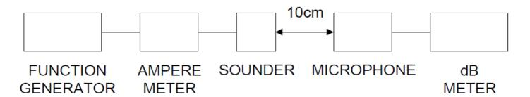
In the measuring test, buzzer is placed as follows:
