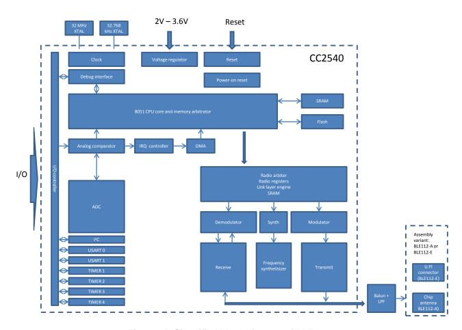
Figure 15: Simplified block diagram of BLE113
