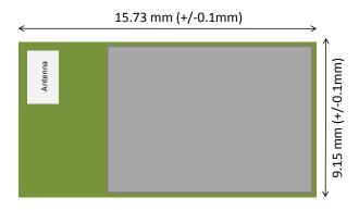
Figure 6: Physical dimensions (top view)
