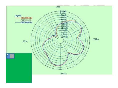
Figure 2: Radiation pattern of BLE113, top view
