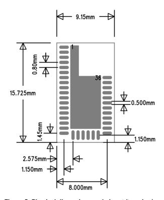
Figure 5: Physical dimensions and pinout (top view)
