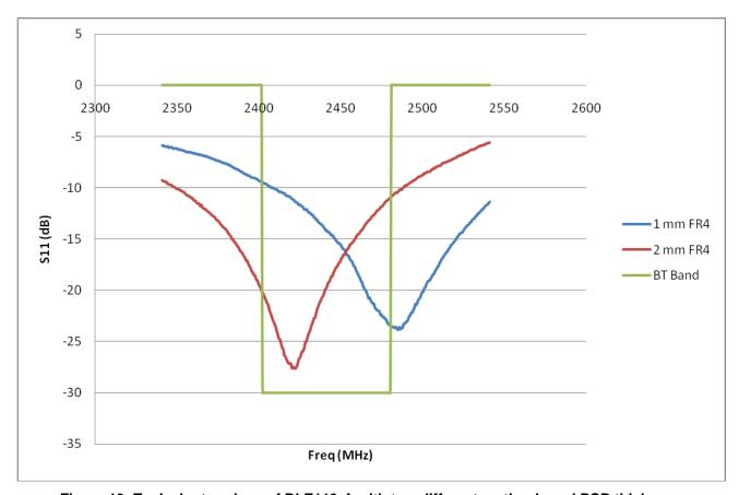
Figure 13: Typical return loss of BLE113-A with two different mother board PCB thickness
