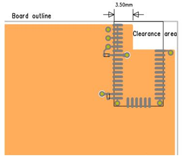
Figure 12: Recommended layout for BLE113-A
