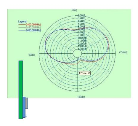
Figure 4: Radiation pattern of BLE113, side view
