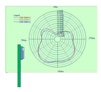
Figure 3: Radiation pattern of BLE113, front view
