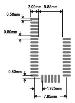
Figure 8: Recommended land pattern for BLE113-A
