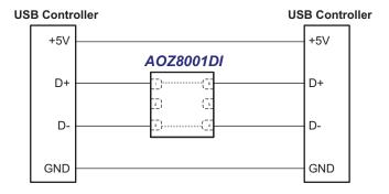
Figure 1. USB 2.0 High Speed Port
