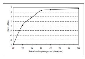
4.6 The Normalized Antenna Gain Chart (For Example:1585MHz)
