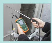
New sensor technology delivers major improvements in durability and ATC (Automatic Temperature Compensation) for accurate in-duct Air Velocity measurements with changing air temperatures. Telescoping probe with ruler label ensures that measurements are made in the center of the duct even if out of reach. Ergonomic directional handle and anti-rotation sensor confirms that probe direction and airflow direction are aligned for confident readings.
