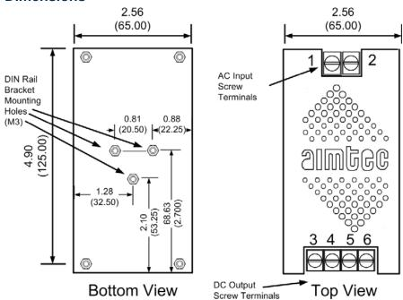
Dimensions: inch (mm) Case Tolerance: ±0.05 (±1.30)
