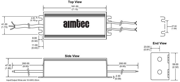
Measurements in Millimeters (inch) Case Tolerance:  $\pm 0.5$  ( $\pm 0.02$ )
