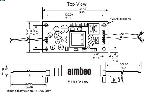
NOTE: to adjust the output current connect a 20K Ohm pot between blue and white wire
