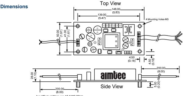
Input/Output Wires are 18 AWG 20cm
