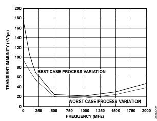
Figure 24. Transient Immunity (Sinusoidal Transients), 100°C Ambient Temperature
