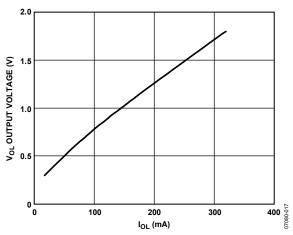
Figure 10. Typical  $V_{OL}$  vs.  $I_{OL}$  ( $V_{DD1} = 5$  V,  $V_{DDB}$ ,  $V_{ISO} = 12$  V to 18 V)
