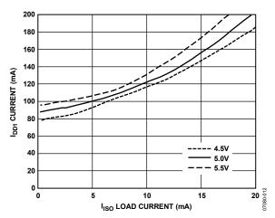
Figure 5. Typical V<sub>DD1</sub> Supply Current vs. V<sub>ISO</sub> External Load Current
