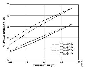
Figure 11. Typical Propagation Delay vs. Temperature
