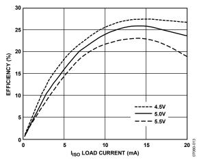
Figure 6. Typical V<sub>ISO</sub> Supply Efficiency vs. V<sub>ISO</sub> External Load Current
