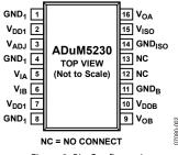
Figure 3. Pin Configuration
