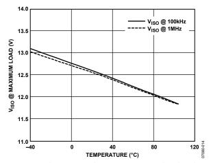
Figure 7. Typical  $V_{\rm ISO}$  Output Voltage at Maximum Combined Load Over Temperature
