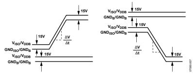
Figure 20. Common-Mode Transient Immunity Waveforms—Between Outputs
