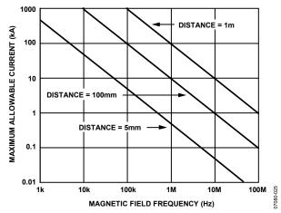
Figure 18. Maximum Allowable Current for Various Current-to-ADuM5230 Spacings
