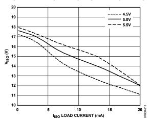
Figure 4. Typical  $V_{\rm ISO}$  Supply Voltage vs.  $I_{\rm ISO}$  External Load Current
