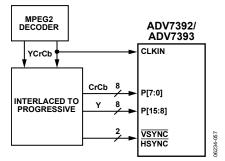
*Figure 59. ED/HD-SDR Example Application*
