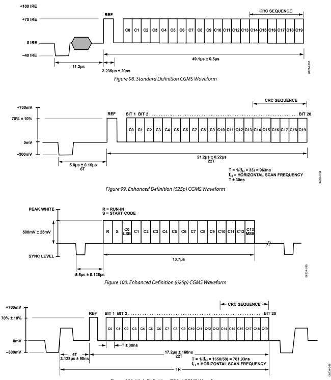
Figure 101. High Definition (720p) CGMS Waveform
