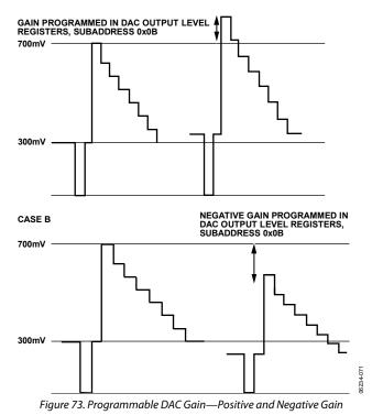
The range of this feature is specified for  $\pm 7.5\%$  of the nominal output from the DACs. For example, if the output current of the DAC is 4.33 mA, the DAC gain control feature can change this output current from 4.008 mA (-7.5%) to 4.658 mA (+7.5%).
