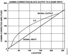
Figure 74. Signal Input (Ramp) and Signal Output for Gamma 0.5
