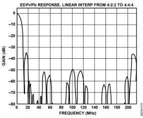
Figure 21. ED 8× Oversampling, PrPb Filter (Linear) Response
