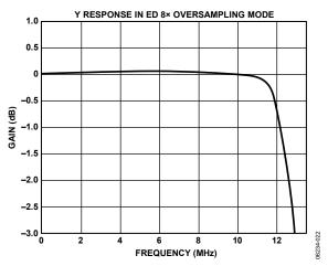
Figure 24. ED 8× Oversampling, Y Filter Response (Focus on Pass Band)
