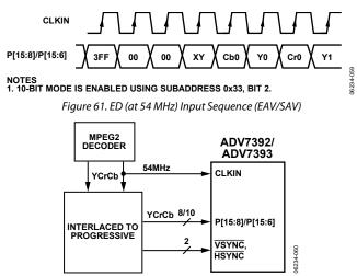
Figure 62. ED (at 54 MHz) Example Application
