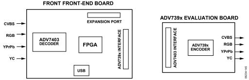
Figure 147. ADV739x Front-End and Back-End Evaluation Boards
