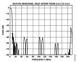
Figure 22. ED 8× Oversampling, PrPb Filter (SSAF™) Response
