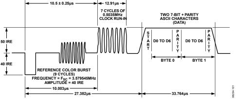
Figure 106. SD Closed Captioning Waveform, NTSC
