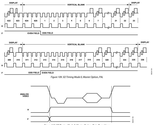
Figure 110. SD Timing Mode 0, Master Option, Data Transitions
