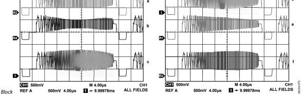
Figure 77. ED/HD Sharpness Filter Control with Different Gain Settings for ED/HD Sharpness Filter Gain Values
