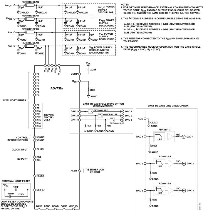
Figure 96. ADV739x (LFCSP) Typical Applications Circuit
