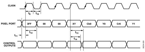
Figure 11. ED (at 54 MHz) Input, 8-/10-Bit 4:2:2 YCrCb (EAV/SAV), Input Mode 111
