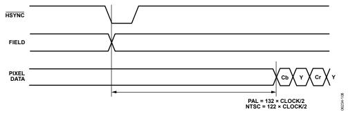
Figure 113. SD Timing Mode 1, Odd/Even Field Transitions (Master/Slave)
