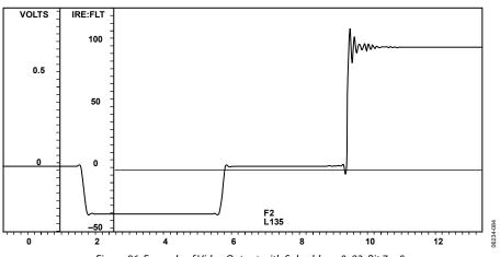
Figure 86. Example of Video Output with Subaddress 0x82, Bit 7 = 0
