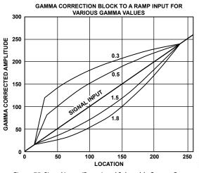
Figure 75. Signal Input (Ramp) and Selectable Output Curves
