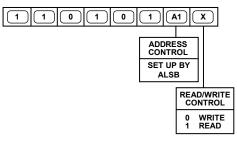
Figure 47. ADV7390/ADV7392 I<sup>2</sup>C Slave Address
