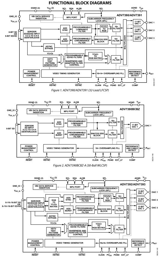
Figure 3. ADV7392/ADV7393 (40-Lead LFCSP)
