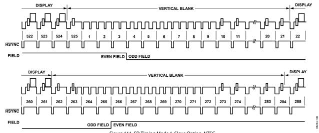
Figure 111. SD Timing Mode 1, Slave Option, NTSC
