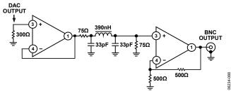
Figure 92. Example of Output Filter for HD, 4× Oversampling
