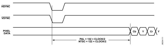
Figure 116. SD Timing Mode 2, Even-to-Odd Field Transition (Master/Slave)
