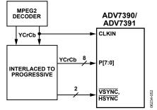
Figure 54. ED/HD-DDR Example Application
