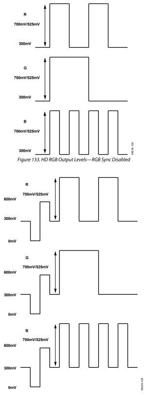
Figure 134. HD RGB Output Levels—RGB Sync Enabled
