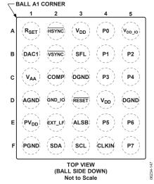
Figure 20. ADV7390BCBZ-A Pin Configuration
