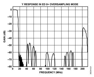
Figure 23. ED 8× Oversampling, Y Filter Response
