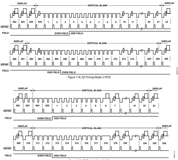
Figure 119. SD Timing Mode 3, PAL
