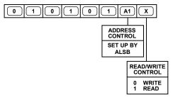
Figure 48. ADV7391/ADV7393 I<sup>2</sup>C Slave Address
