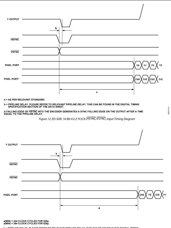
b = PIPELINE DELAY. PLEASE REFER TO RELEVANT PIPELINE DELAY. THIS CAN BE FOUND IN THE DIGITAL TIMING SPECIFICATION SECTION OF THE DATA SHEET.
