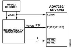
Figure 60. ED/HD-DDR Example Application
