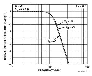
Figure 12. Large Signal Frequency Response for Various Supplies
