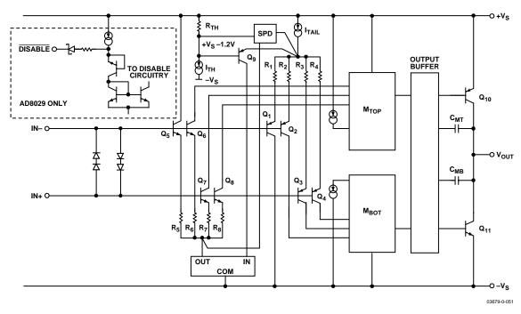
Figure 50. Simplified Schematic
