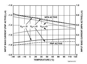
Figure 38. Input Bias Current vs. Temperature
