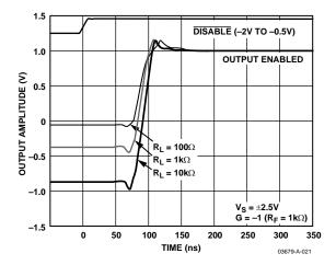
Figure 48. AD8029 DISABLE Turn-On Timing
