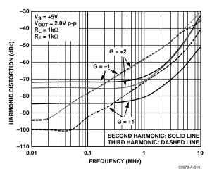
Figure 21. Harmonic Distortion vs. Frequency and Gain
