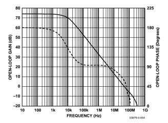
Figure 15. Open-Loop Gain and Phase vs. Frequency
