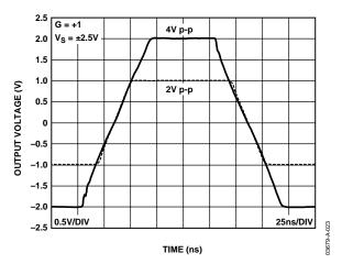
Figure 26. Large Signal Transient Response
