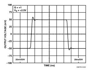
Figure 25. Small Signal Transient Response
