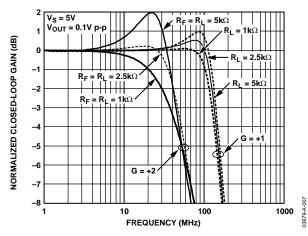
Figure 55. Frequency Response for Various Feedback/Load Resistances
