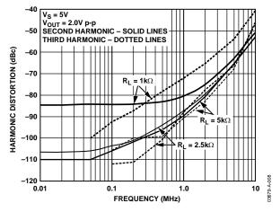
Figure 53. Gain of 1 Distortion
