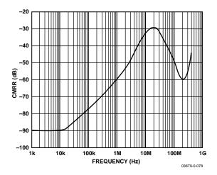
Figure 32. Common-Mode Rejection Ratio vs. Frequency
