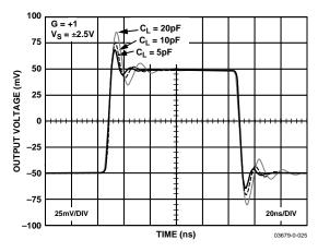
Figure 28. Small Signal Transient Response with Capacitive Load
