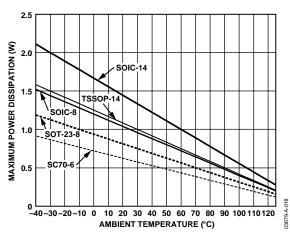
Figure 6. Maximum Power Dissipation
