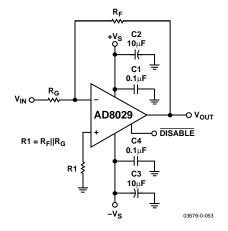
Figure 52. Wideband Inverting Gain Configuration
