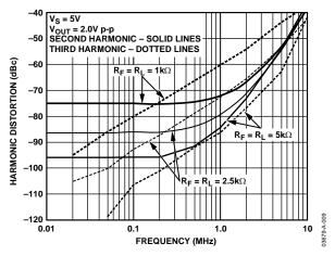
Figure 54. Gain of 2 Distortion
