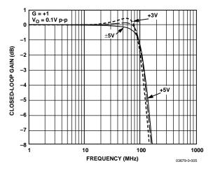
Figure 8. Small Signal Frequency Response for Various Supplies
