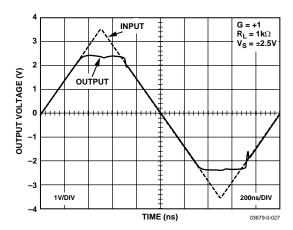
Figure 30. Input Overdrive Recovery
