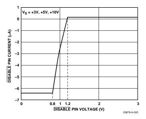
Figure 49. AD8029 DISABLE Pin Current vs. DISABLE Pin Voltage
