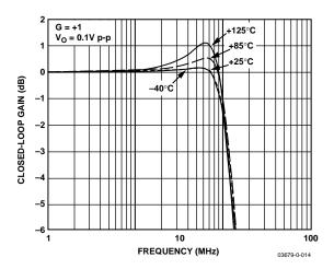
Figure 17. Small Signal Frequency Response vs. Temperature
