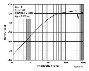
Figure 33. AD8029 Off-Isolation vs. Frequency
