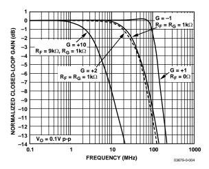
Figure 7. Small Signal Frequency Response for Various Gains
