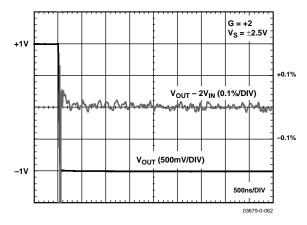
Figure 31. Long-Term Settling Time
