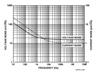
Figure 24. Voltage and Current Noise vs. Frequency
