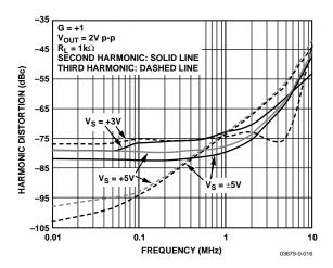
Figure 19. Harmonic Distortion vs. Frequency and Supply Voltage
