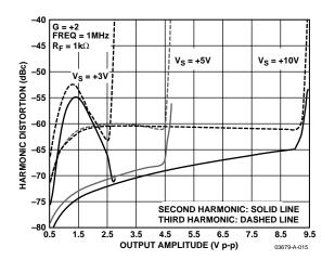
Figure 20. Harmonic Distortion vs. Output Amplitude
