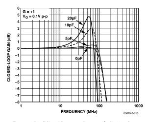
Figure 13. Small Signal Frequency Response for Various CLOAD
