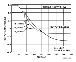
Figure 47. AD8029 DISABLE Turn-Off Timing
