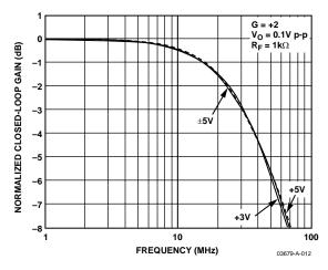
Figure 11. Small Signal Frequency Response for Various Supplies
