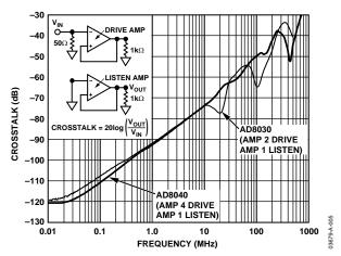
Figure 36. AD8030/AD8040 Crosstalk vs. Frequency
