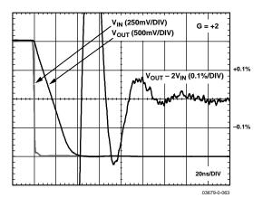
Figure 34.0.1% Short-Term Settling Time
