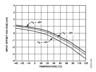
Figure 41. Input Offset Voltage vs. Temperature
