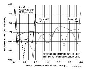
Figure 23. Harmonic Distortion vs. Input Common Mode Voltage
