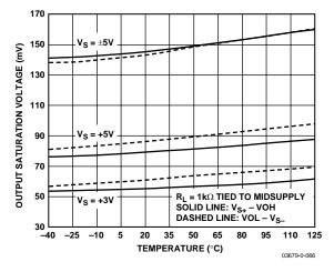
Figure 42. Output Saturation Voltage vs. Temperature
