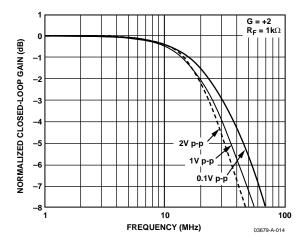
Figure 14. Frequency Response for Various Output Amplitudes
