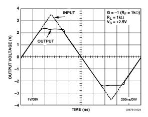
Figure 27. Output Overdrive Recovery
