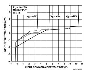
Figure 40. Input Offset Voltage vs. Input Common-Mode Voltage
