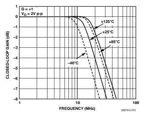
Figure 18. Large Signal Frequency Response vs. Temperature
