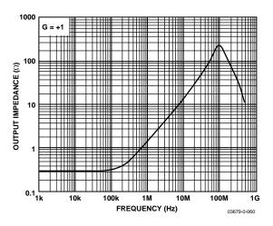
Figure 45. Output Impedance vs. Frequency, Enabled
