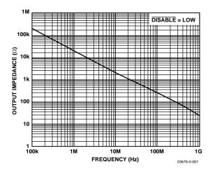
Figure 43. AD8029 Output Impedance vs. Frequency, Disabled
