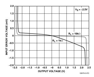
Figure 46. Input Error Voltage vs. Output Voltage
