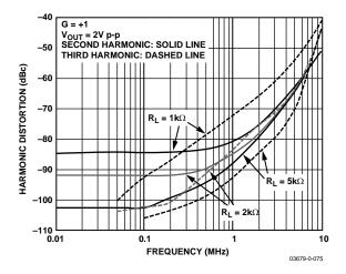
Figure 22. Harmonic Distortion vs. Frequency and Load
