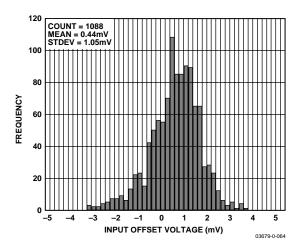
Figure 42. Input Offset Voltage Distribution
