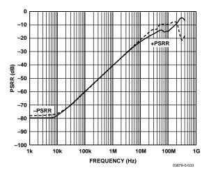
Figure 35. PSRR vs. Frequency
