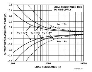
Figure 44. Output Saturation Voltage vs. Load Resistance
