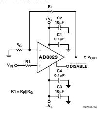
Figure 51. Wideband Non-inverting Gain Configuration
