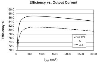
Circuit for 42 V step down to 3.3 V at 3 A. Efficiency data from circuit shown in left panel. Data is for reference only.
