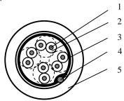
1. Conductor AWG24 (7xAWG32) tinned Cu
