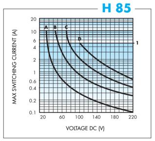
Breaking capacity for DC1 load.
