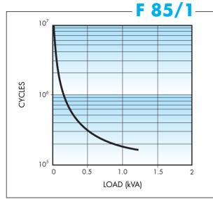
DC contact life vs AC1 load. 4 CO types (5 A)
