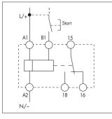
\* The functions with external start (B1) may be activated using a different voltage from that used for the supply voltage.
