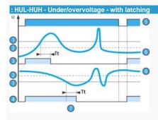
If "with memory" mode has been selected, the relay opens and stays in this position when threshold crossing is detected. The power supply must be disconnected to reset the product.
