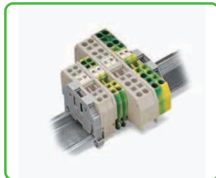
End and intermediate plate In order to meet creepage and clearance requirements for Ex e applications, it is necessary to insert an end or intermediate plate between a through and a ground conductor terminal block.
