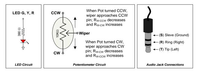
Figure 2. Digilent myProto circuits and breadboard device connections.
