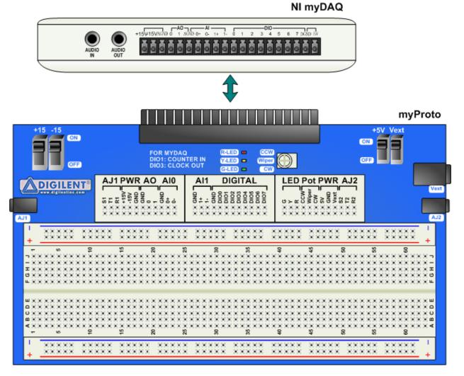
Figure 1. Connecting Digilent myProto to the NI myDAQ.
