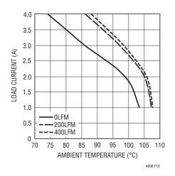
Figure 10.  $5V_{\text{IN}}$  to 2.5 $V_{\text{OUT}}$  No Heat Sink
