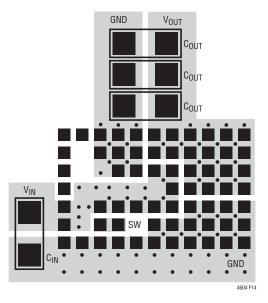
Figure 14. Recommended PCB Layout
