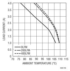
Figure 6.  $5V_{\text{IN}}$  to 1.2V\_{\text{OUT}} No Heat Sink
