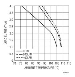
Figure 11.  $5V_{\mbox{\scriptsize IN}}$  to  $2.5V_{\mbox{\scriptsize OUT}}$  with Heat Sink
