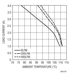
Figure 9. 3.3  $V_{\text{IN}}$  to 1.2  $V_{\text{OUT}}$  with Heat Sink
