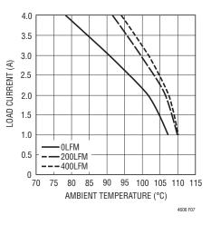
Figure 7.  $5V_{\text{IN}}$  to 1.2 $V_{\text{OUT}}$  with Heat Sink
