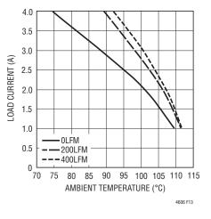
Figure 13. 3.3  $V_{\text{IN}}$  to 2.5  $V_{\text{OUT}}$  with Heat Sink
