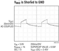
**Output Voltage Waveform When**
