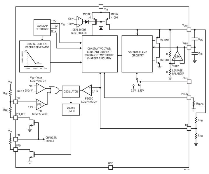
Figure 1. LTC4425 Block Diagram
