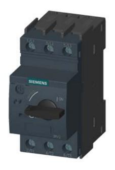
CIRCUIT-BREAKER SZ S00, FOR MOTOR PROTECTION, CLASS 10, A-RELEASE 9..12.5A, N-RELEASE 163A, SCREW CONNECTION, STANDARD SW. CAPACITY
