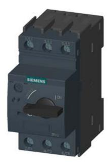
CIRCUIT-BREAKER SZ S00, FOR MOTOR PROTECTION, CLASS 10, A-REL. 1.4...2A, N-RELEASE 26A, SCREW CONNECTION, STANDARD SW. CAPACITY
