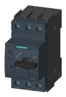
CIRCUIT-BREAKER SZ S00, FOR MOTOR PROTECTION, CLASS 10, A-REL. 0.28...0.4A, N-RELEASE5.2A, SCREW CONNECTION, STANDARD SW. CAPACITY
