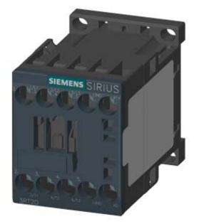
COUPLING RELAY, AC-3, 5.5KW/ 400V , 1NO, DC 24V, 0.7...1.25\*US, W. INTEGRA. SUPPRESSOR DIODE, SZ S00, SCREW TERMINAL
