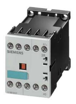
COUPLING RELAY, AC-3 5,5 KW/400 V, 1 NO, DC 24 V, 0.7...1.25\*US, W. VARISTOR, 3-POLE, SIZE S00, SCREW CONNECTION
