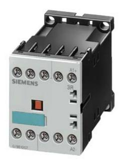
COUPLING RELAY, AC-3 5,5KW/400 V, 1 NO, DC 24 V, 0.7...1.25\*US, W.DIODE 3-POLE, SIZE S00, SCREW CONNECTION
