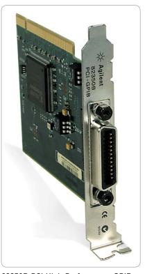
82350B PCI High-Performance GPIB Interface Card
