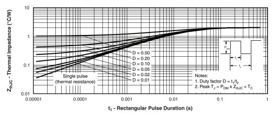
Fig. 4 - Maximum Thermal Impedance  $Z_{thJC}\ Characteristics$
